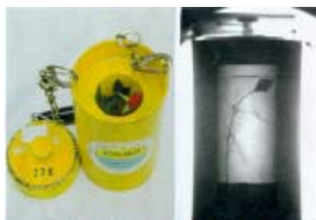
Neutrons penetrate deep into matter. Neutron radiography of a rose inside a thick lead container
